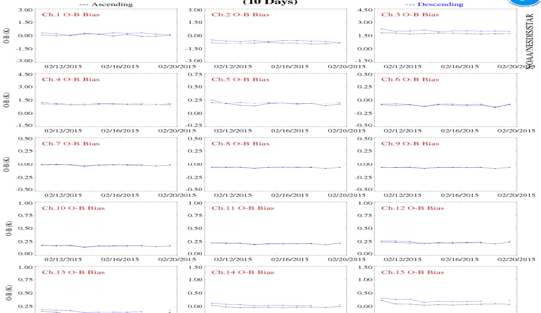
S-NPP ATMS Daily Global Mean Bias Time Series (IDPS TDR - CRTM SIM) (10 Days)
